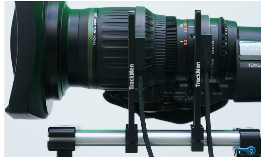
Illustration 1: External encoders installed
