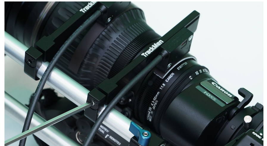
Illustration 9: Fasten the mount screw firmly
