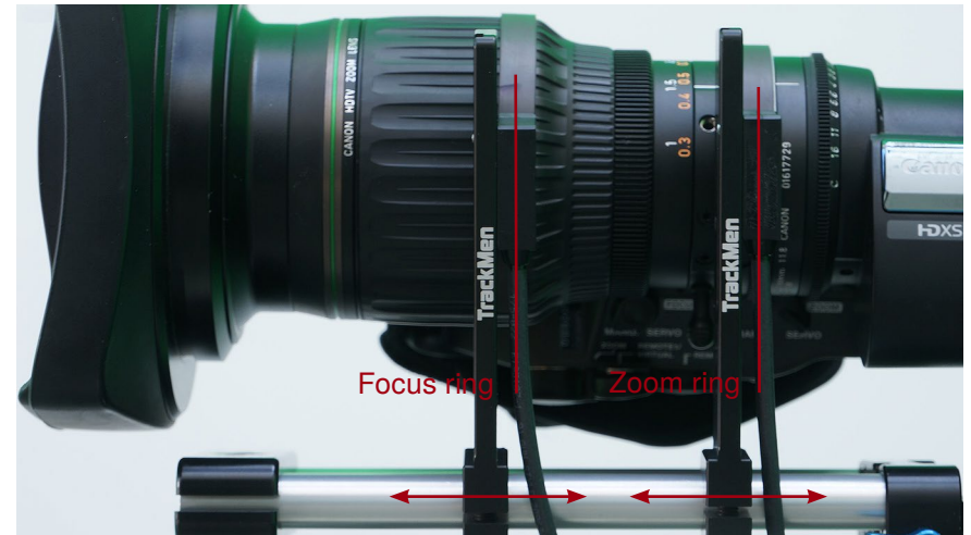
Illustration 4: Find the position of the zoom/focus rings along the accessory rod
