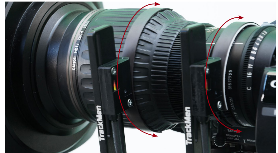
Illustration 12: Initialization; turn both rings the whole way after system start
