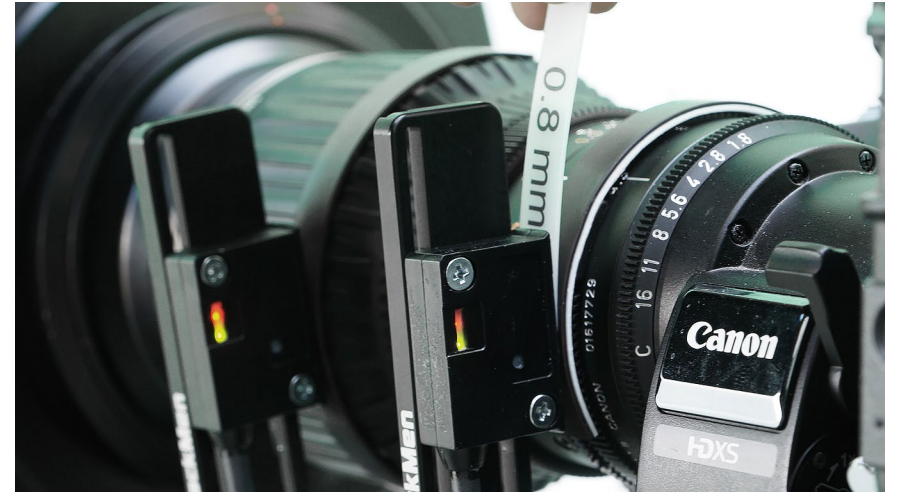
Illustration 8: Fix the encoder in the correct distance to the tape
