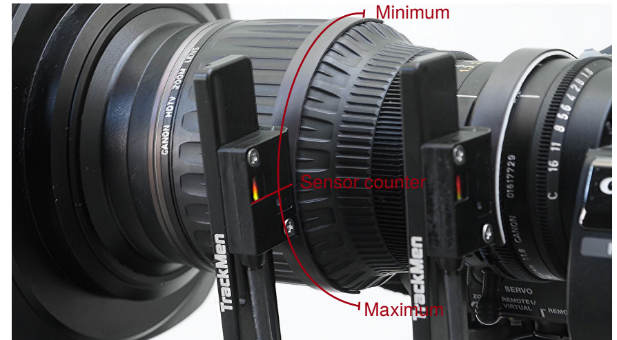
Illustration 6: Evaluate the respective ring range that needs to be covered by the tape
