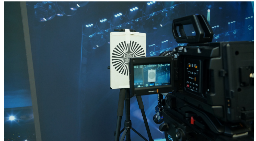
Siemens star placed in front of the camera
