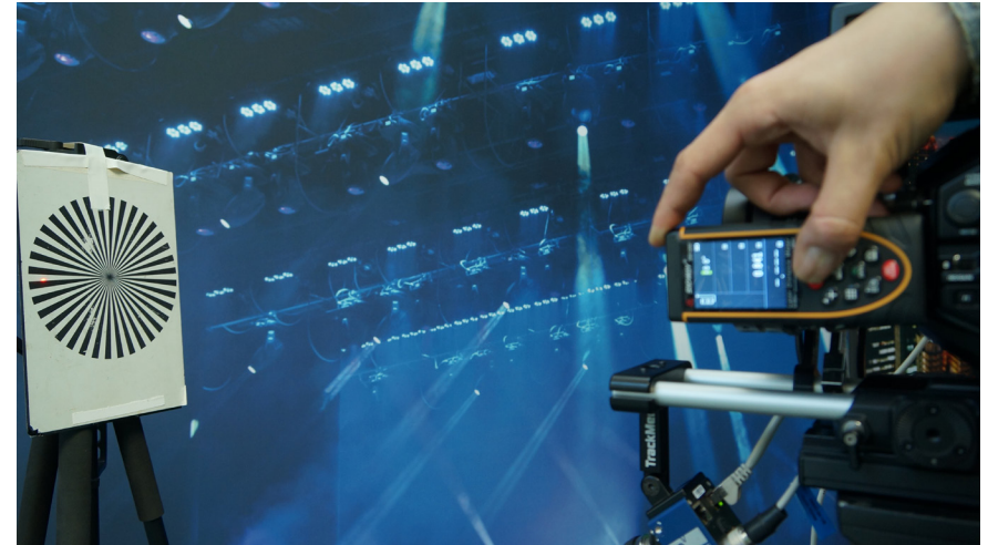
Focus the object and measure the distance while reading the encoder value from the System log.
